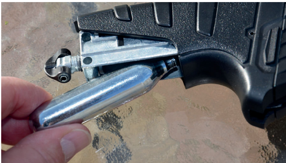
ABOVE LEFT: Inserting a fresh 12g CO2 capsule
